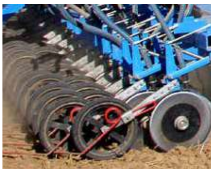
The double disc coulters
