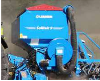
The hydraulically driven fan
